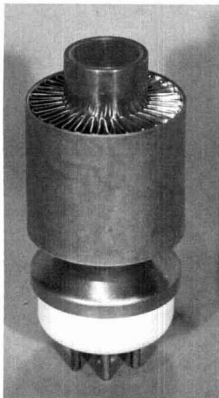
fig. 3. The new EIMAC 3CX1200A7 high- \mu power triode.
